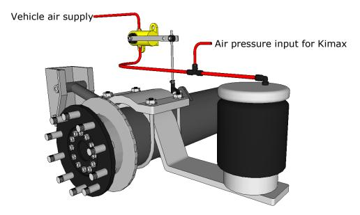
In order to make the Kimax 2 Radio work properly on your vehicle, you need to teach the instrument how to calculate different loads. So before you can rely on your new on-board scale, each axle has to be calibrated after the installation. The calibration is carried out by weighing each axle of the vehicle on a weighing bridge. While your truck is standing on the weighing bridge you must give in the empty weight (LO) and loaded weight (HI), when the vehicle is empty or loaded respectively.
