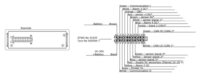
The connections above marked with `\*' are only present if the connection is required by the part number for a given instrument. This example is for a fully featured device.
