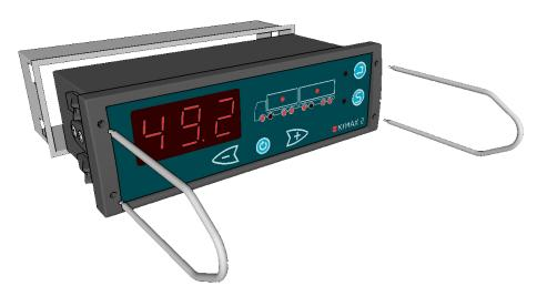
In order to replace the Kimax 2 Radio, you need to use the two belonging forks for releasing the snaps before you can pull the instrument out of the frame.
