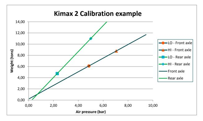
The air pressure is measured on the right and left side of each axle and routed to the Kimax instrument, to obtain the most accurate weighing results under different circumstances.
