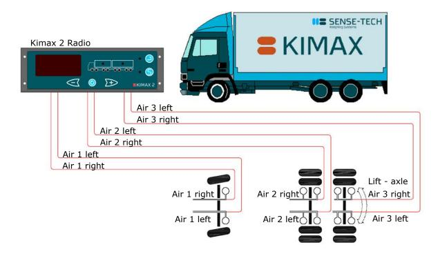
When your lift-axle is engaged, the pressure in air 3 left equals air 2 left and the pressure in air 3 right equals air 2 right, axle 2 and 3 share the weight of the rear of your vehicle.
