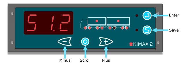
By use of the buttons 0, 2 and 2, you can display the individual weight of each axle, the load you are carrying and the total weight of your vehicle.
